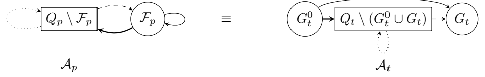
Figure 2.1: Construction of \mathcal{A}_t from \mathcal{A}_p . Similar node shape represents equivalent state sets. Similar line style represents equivalent transition function between sets.
